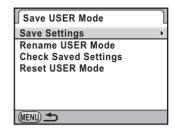
Use the four-way controller (▲▼) to select [USER1] to [USER5] and press the four-way controller (►).
