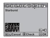
Use the four-way controller (▲▼) to select the parameter and the four-way controller (◀►) to adjust the parameter's value.
