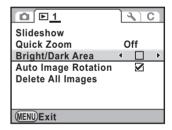
Use the four-way controller (▲ ▼) to select [Auto Image Rotation] and use the four-way controller (◀▶) to select ✓ or □.
