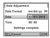
Press the four-way controller (▼) to select [Settings complete].
