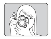
The focus indicator lacktriangle appears and you will hear a beep when the subject comes into focus. (When blinking, the subject is not in focus.)
