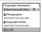
Use the four-way controller (▲ ▼) to select [Photographer] and press the four-way controller (▶).
