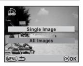
When [Single Image] is selected in Step 3, use the four-way controller (◄►) to select an image to set DPOF settings.
