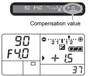
Press the **■** button to check the compensation value after adjustment. Press the **●** button to reset the EV compensation value to 0.0.
