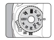
Turn the front e-dial ( ) to adjust the shutter speed.
