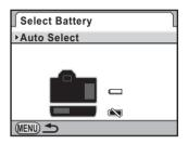
Use the four-way controller (▲ ▼) to select a battery to be prioritized and press the OK button.
