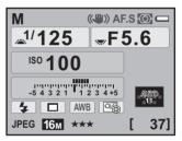
While adjusting the shutter speed or aperture value, the difference from the proper exposure (EV value) is displayed in a bar graph. The proper exposure is set when I is in the middle of the EV bar. If it is towards -, it is underexposed. If it is towards +, it is overexposed. If the value exceeds the range of the EV bar (±5.0), or if the subject is too bright or too dark, the
