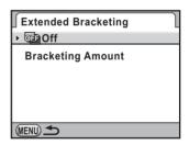
Use the four-way controller (▲ ▼) to select an item and press the OK button.
