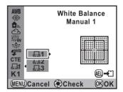
Under the light to measure the white balance, fully display a white sheet of paper in the viewfinder or select a white area as the subject.
