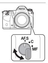
When the shutter release button is pressed halfway and the subject comes into focus, the focus is locked (focus lock) at that position. To focus on another subject, take your finger off the shutter release button first, then press the shutter release button halfway again.
