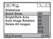
Use the four-way controller (▲ ▼) to select [Bright/Dark Area] and use the four-way controller ( ◀ ▶ ) to select ₩ or □.
