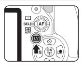
The mirror pops up and a real-time image is displayed on the monitor. Press the **W** button again to exit Live View.
