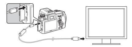
Connect the other end of the HDMI cable to the HDMI input terminal on the AV device.
