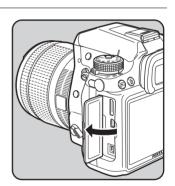
Face the ▲ mark on the DC terminal of the AC adapter towards the ▲ mark on the camera, and connect the DC terminal to the DC input terminal of the camera.
