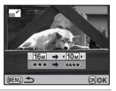
Press the four-way controller (▼) and use the four-way controller (◀▶) to select the quality level.
