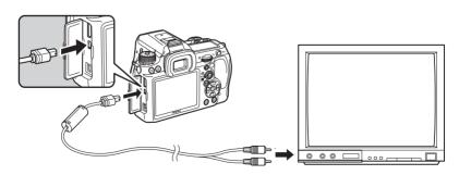
Connect the other end of the AV cable to the video input terminal on the AV device.
