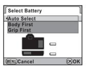
When using AA batteries in the battery grip, use the four-way controller (▲ ▼) to select [AA Battery Type] and press the fourway controller (▶).
