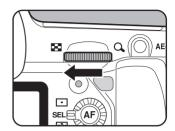
Use the four-way controller (▲▼◀►) to select a folder to delete and press the fill button.
