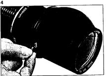
Fig. 4 Loosen the adaptor clamp screw ③ as shown in order to position the porthole at the desired shooting angle. Retighten the screw after the porthole has been adjusted as desired.
