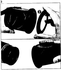
Fig. 3 With lenses having 52mm filter threads, remove the accessory ring ② of the adaptor by unscrewing it counterclockwise, as illustrated. Then, screw the newly exposed 52mm threads of the adaptor into the lens. (Keep the ring nearby when detached to avoid loosing it; be sure to screw it back into place after using the adaptor.)
