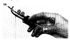
cable release is not inserted (or simply forgotten), the diaphragm will remain open.
