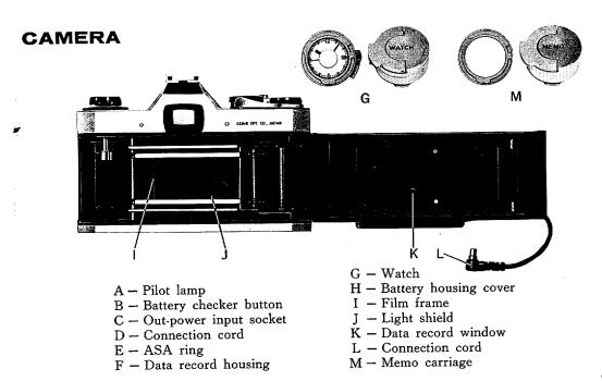
The Pentax DATA II camera has a specially made detachable back with a data record housing. The reading of the watch built in this housing plus written data on the data sheet are projected onto the film for recording at a corner of the film. For photographically recording:
