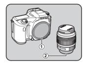
Align the red dots on the camera and the lens, and secure by turning the lens clockwise until it clicks.
