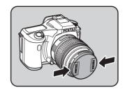
To detach the lens, hold down the lens unlock button (3) and turn the lens counterclockwise
