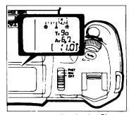
The exposure compensation allows you to deliberately overexpose (brighten) or underexpose (darken) a subject. When the Hyper button [ E ] is depressed, the compensation value and bar graph will be displayed on the LCD panel and in the viewfinder. Select the desired compensation value by turning the Select Dial while holding down the Hyper button.
