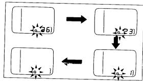
When the roll of film is rewound to its end, [ Q ] blinks and the exposure counter indication disappears, informing you that the back cover may be opened.
