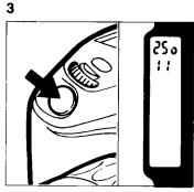
When Using a Manual F-Stop Setting (Move the camera's Main Switch to [ ON ] or [ PICT ] 1
