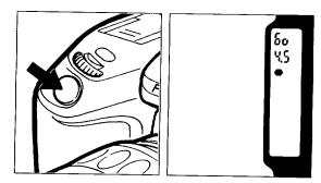
When the shutter release button is depressed halfway down, the shutter speed and aperture setting are displayed in the viewfinder and on the LCD panel. To release the shutter, depress the shutter release button fully. The camera automatically winds the film and the exposure counter indication advances by one. If the subject is dark or backlit, the flash-recommended indicator [ § ] blinks in the viewfinder, advising use of flash. [ § ] also blinks on the LCD panel.
