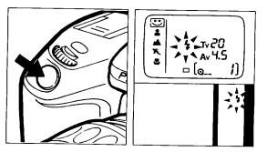
The Flash-Recommended Indicator [5] When a subject is shot in dark or in a backlit situation in the Programmed AE (including the Picture Mode) or Aperture-Priority AE mode, the flash-recommended indicator blinks in the viewfinder and on the LCD panel to recommend the use of the built-in flash. In the Shutter-Priority AE Mode, the flash-recommended indicator appears only when a subject is shot in a backlit situation
