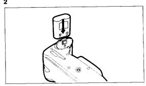
Insert the battery, making sure the plus/minus markings (+/-) match the diagrams inside the battery compartment. Then, reinstall the battery chamber cover.
