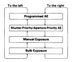
With the lens aperture ring at "A" (auto), moving the camera's Main Switch to [ ON ] (full-feature position) lets you select any of the available exposure modes other than the Picture Mode, without having to turn the aperture ring to a manual f-stop setting.
