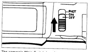
The camera's Main Switch has three positions.
