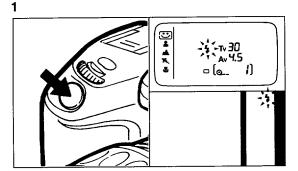
When using the camera's built-in flash in a dark or backlit situation, the camera automatically chooses an optimum combination of shutter speed and aperture according to the subject brightness, allowing you to take a flash photograph with ease.
